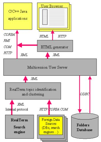
RealTerm is implemented as a server application or through an ASP, which connects to thin clients (web browsers) or other applications through HTTP or other network protocols passing XML or HTML. The *Multi-User Server* monitors connections with multiple users coordinating requests and data traffic. It generates XML which then is transformed into HTML (if necessary) using XSLT.
